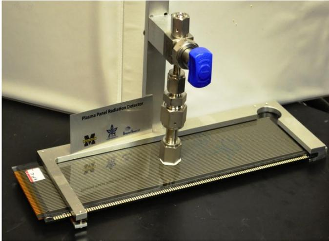
Fig. 3. PPS “refillable” test panel.
