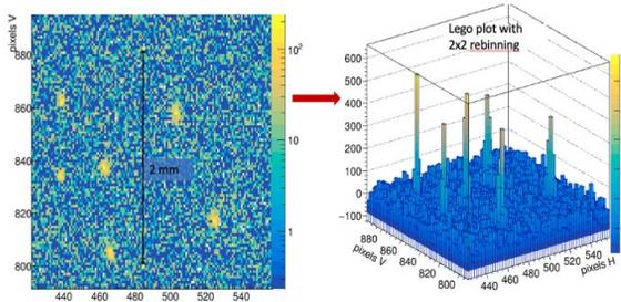
Figure 4: Individual <sup>86</sup>Kr hits on HM type scintillator. Camera frame exposure time = 1 s, beam rate ~5-10 pps.
